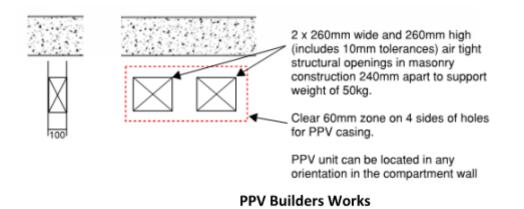
It is recommended the two structural openings are of blockwork or solid infill construction so as to support a weight of 50kgs. Where the wall cannot support this weight, drop rods can be utilised to support the unit.
