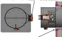
38mm long drywall screws to affix installation plate to metal frame within drywall (see 6.11)
