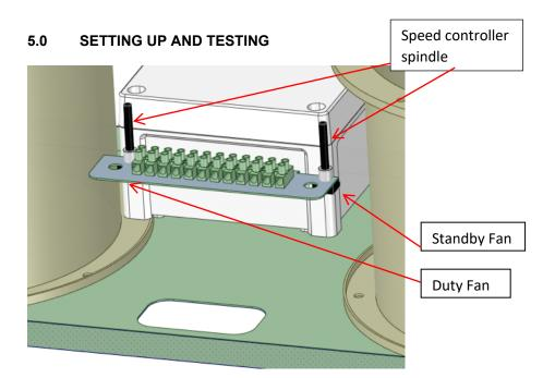
The duty and standby fans are each fitted with a speed control module. These are located adjacent to the fan and is adjusted using the black spindle which is mounted on either side of the terminal connection block as shown in the picture above. Do not bend the spindle.
